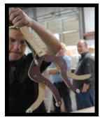
Team 1987 uses a somewhat unorthodox method to pick up tubes from the playing field and hang them on the scoring grid. The gripper device grabs tubes from the center rather than from the edge of the tube. The grippers are made from aluminum or a poly-
